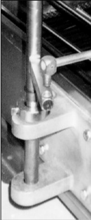
Figure 1-4. Connecting the Swing Connecting Rod.
