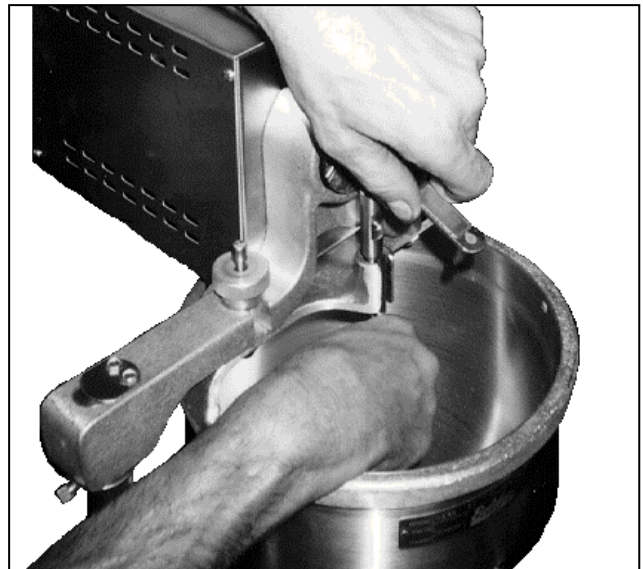
Figure 1-7. Installing the Plunger.
