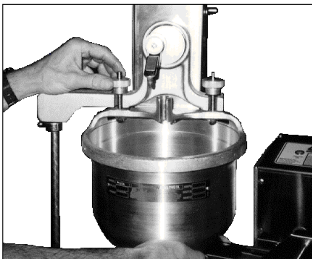
Figure 1-6. Mounting the Hopper.
