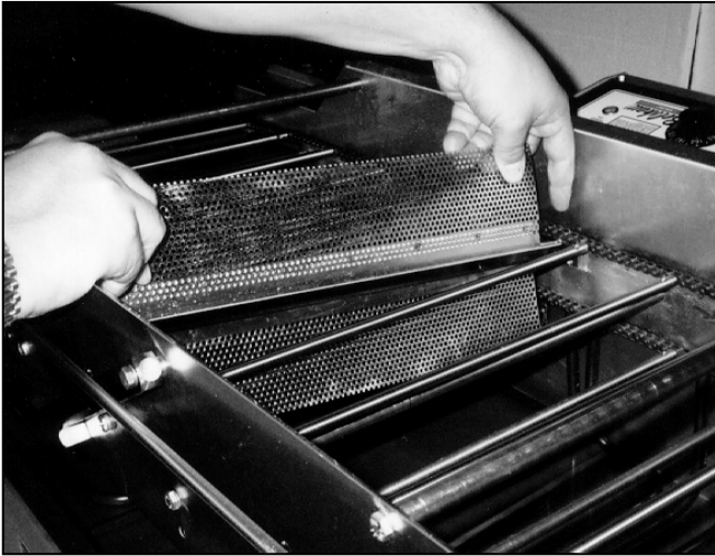
Figure 4 Removing the Turner
