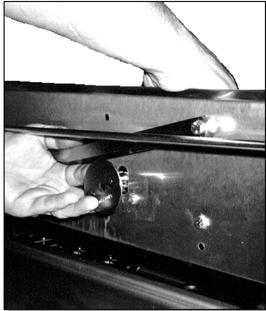
Figure 3 Removing the Turner Cam
